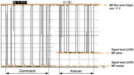
MP-Bus levels OK: Signal level >11 V
