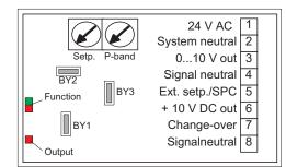
Jumper BY1 Closed = I-time is 2 minutes (delivery setting)
